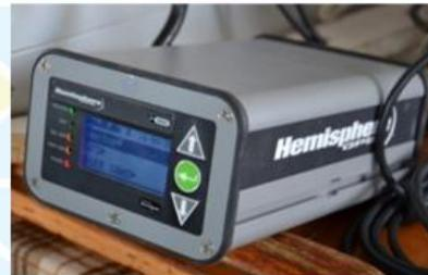
Leica GS08 RTK GNSS System (left image) and Hemisphere VS101 GPS (right image)
