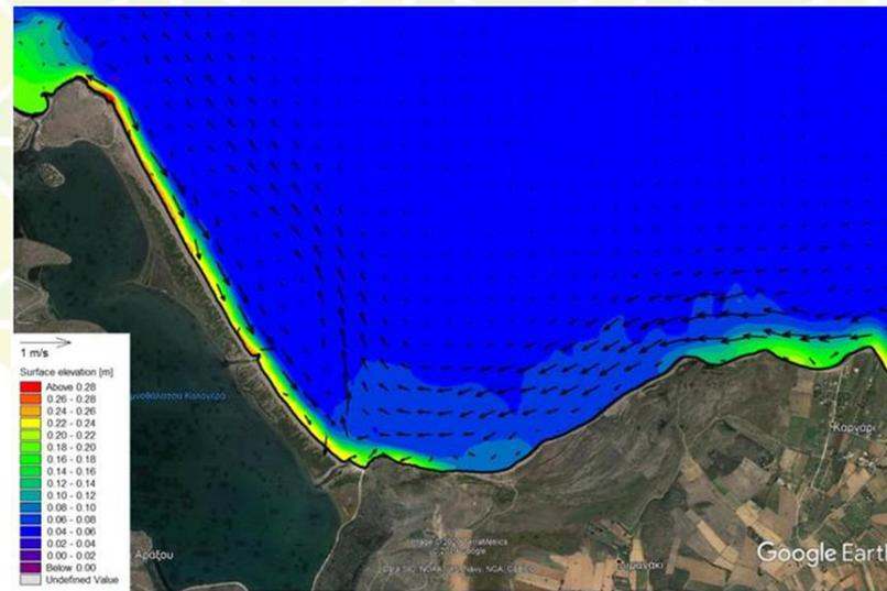
Wave-generated currents (vectors) and wave setup due to northeastern waves in the coastal zone of subregion 1
