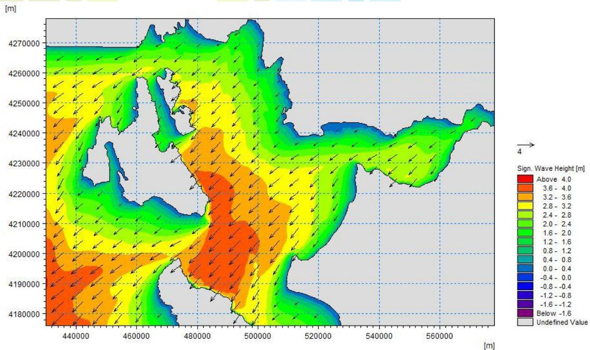
**Figure 27:** Wave height, velocity and direction distribution in the area of the Ionian Sea west of the Gulf of Patras due to the action of northeastern winds.
