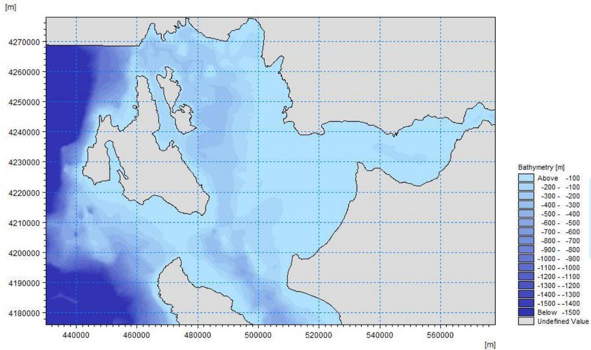
**Figure 256:** The bathymetric computational mesh of the Ionian Sea west of the Gulf of Patras, which was used the numerical in simulations of wind-induced wave generation, growth and propagation.
