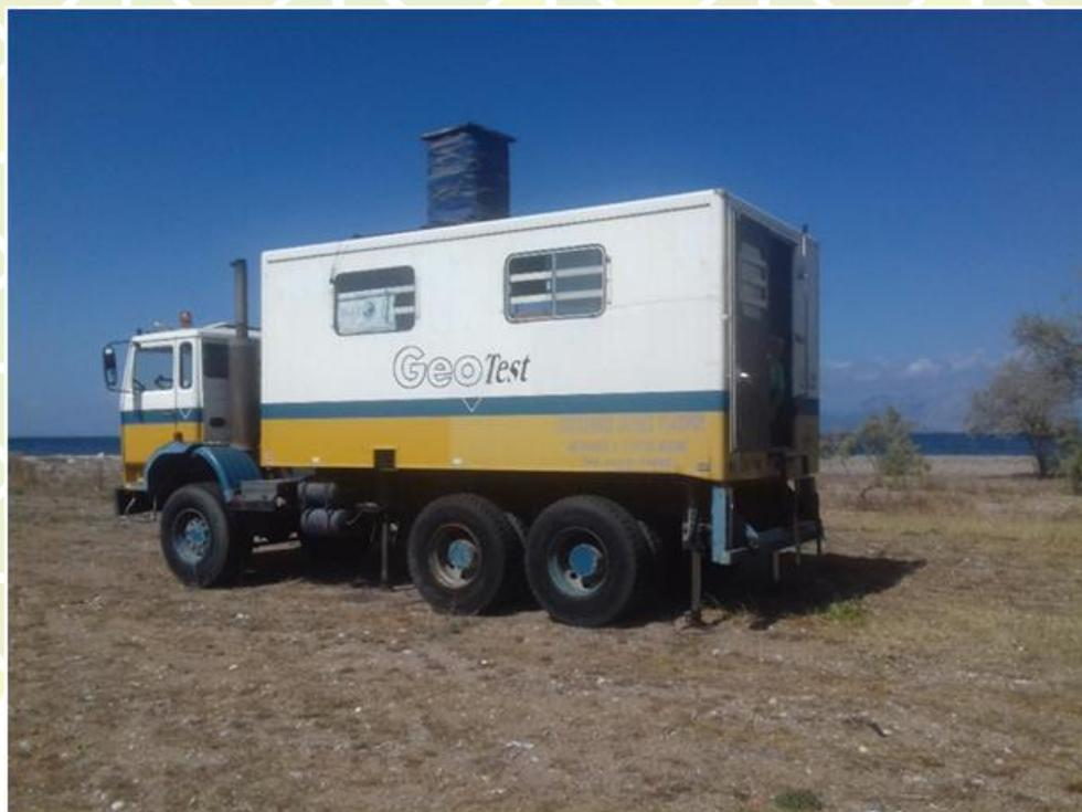
**Figure 3.26:** The static penetrometer 20tn by Gouda/GeomilB.V, on a 6x6 Volvo / Terberg wheeled truck used in the CPT survey
