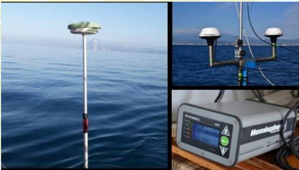
**Figure 3.16:** Leica GS08 RTK GNSS System (left image) and Hemisphere VS101 GPS (right image)
