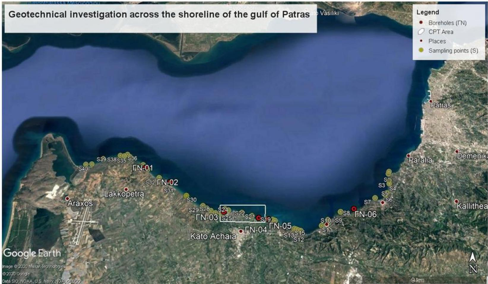
**Figure 3.23:** Google-Earth map representing the geotechnical operations performed along the shoreline of the gulf of Patras (borehole drilling: ΓN, CPT tests and sampling points for sediment analysis: S)
