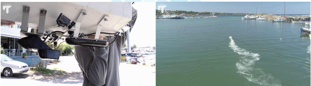
**Figure 3.10:** (a) The bottom of the USV where the SONAR, the Side Scan Sonar and the cameras are placed and (b) USV operation in the Alikes fishery port
