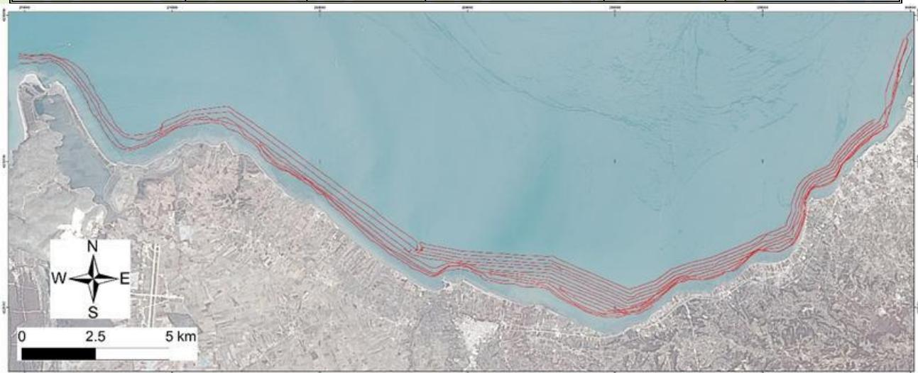
**Figure 3.21:** Map of the gulf of Patras presenting the vessel's bathymetric survey track lines
