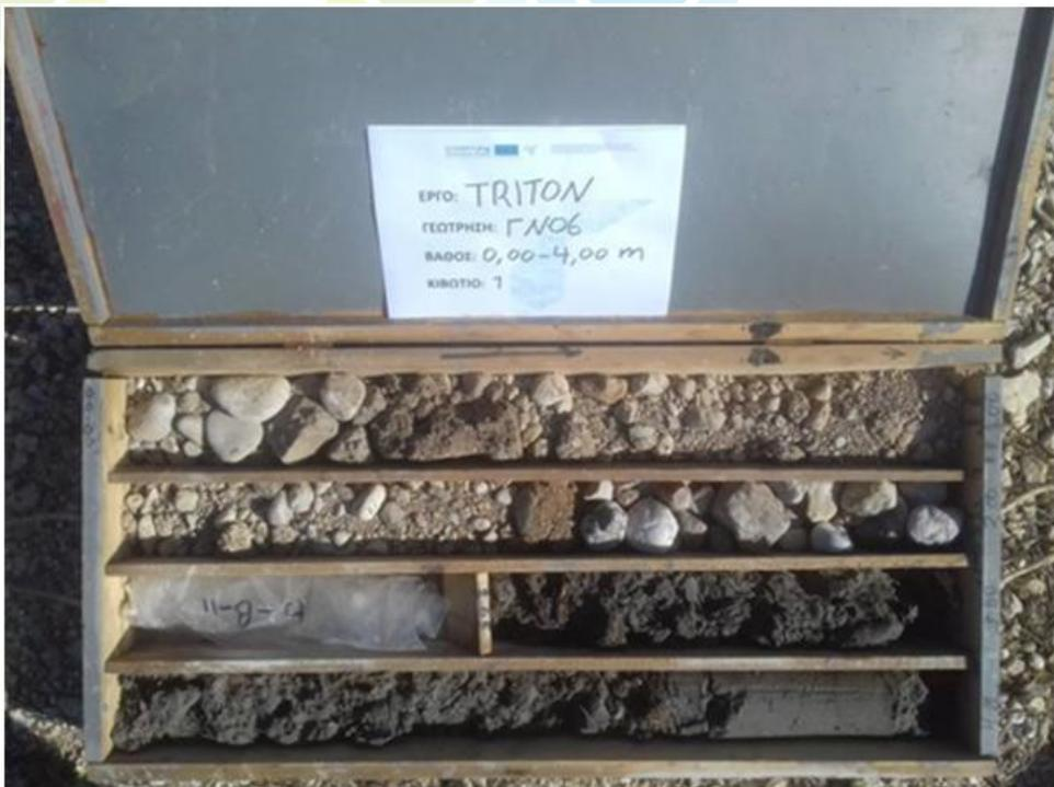
**Figure 3.25:** Log box with soil core samples from borehole ΓN-06 at a depth 0-4m
