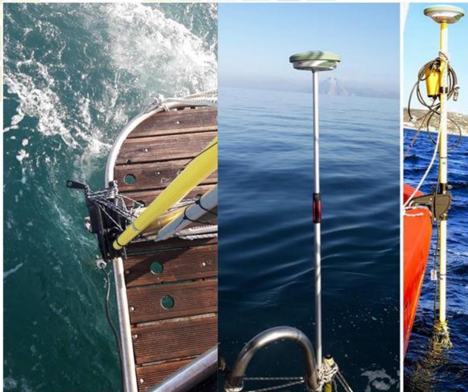
*Figure 3.20: The Hydrolite TM echosounder associated with an RTK GPS installed on top of it*
