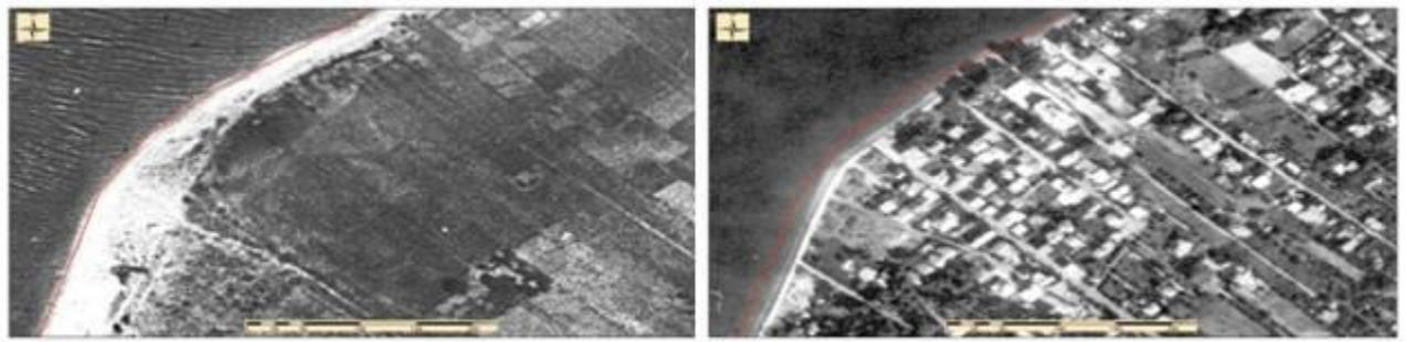
**Figure 3.7:** An example from the 1945 air photo (left image) and 1996 air phot (right image) orthomosaic of the broader coastline northeast of Patras (in red color is the 1945 shoreline). The shoreline retreat is evident
